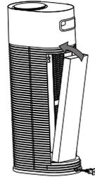
2. Install the rear cover and press the buckle until you hear the "ba" sound to prove that the lock is locked.
